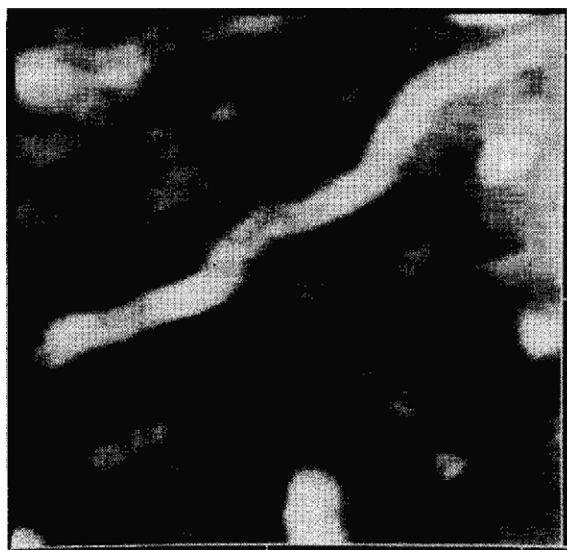
Fig. 13. 215 nm × 215 nm raw data AFM image (tapping mode) of retinal-β-CD complex deposited on a silicon (1 0 0) wafer. The bar indicates 100 nm. Reprinted from Botella et al. (1996).
