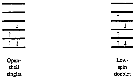
Figure 3 Orbital energy level diagrams for the open-shell singlet and low-spin doublet cases.
