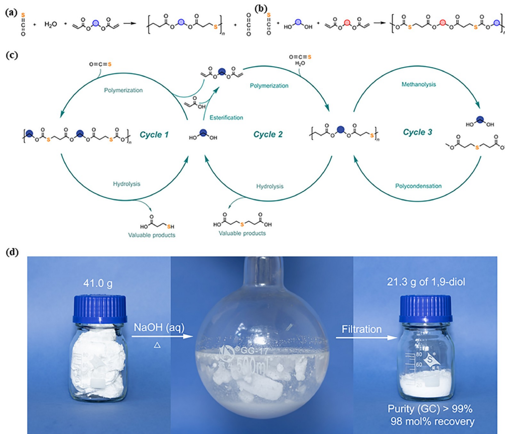
Figure 20 (a) Synthesis of polymers with in-chain ester and thioether groups from polymerization of COS, H 2 O, and diacrylates. (b) Synthesis of polymers with in-chain ester and thiocarbonate groups from polymerization of COS, diols, and diacrylates. (c) Schematic diagram of the chemical recycling of the polymers: Cycle 1 shows the cycle of the second system; Cycles 2 and 3 show the cycle of the first system. (d) Chemical recyclability of obtained polymers. Reproduced from Ref. [113] with permission. Copyright 2023 Wiley-VCH GmbH (color online).
